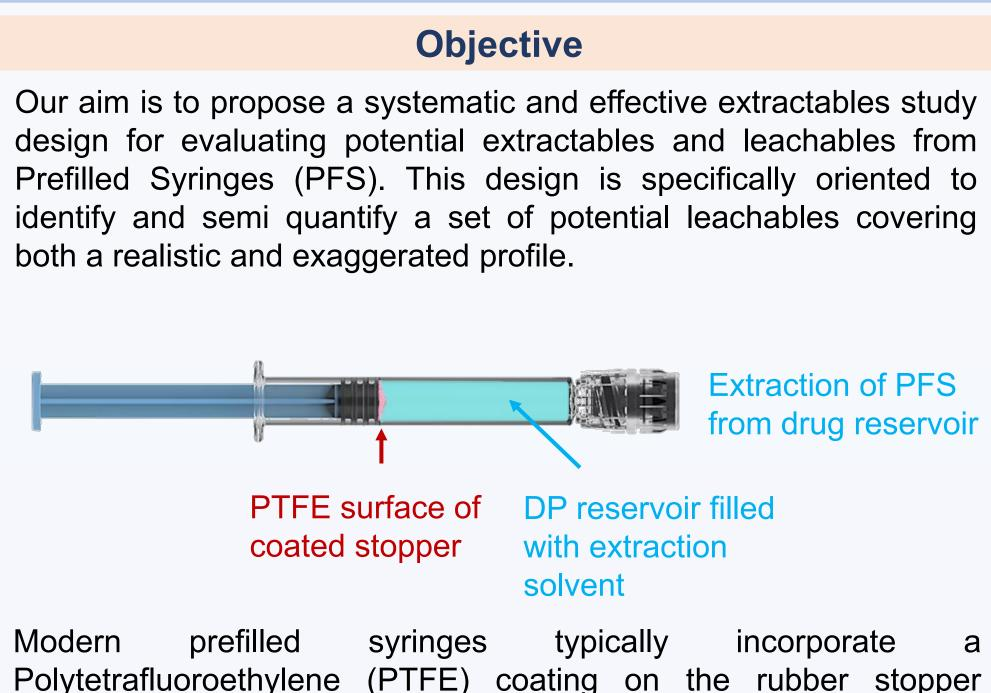
Polytetrafluoroethylene (PTFE) coating on the rubber stopper surface that directly contacts the drug product. Extractables studies that indiscriminately extract such stoppers may overlook the effect of this protective coating, leading to an overestimation of the number and concentrations of extractables.
